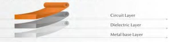
Double-Sided PCB with Aluminum Substrate
