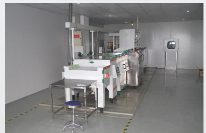
PCB Cleaning Line
